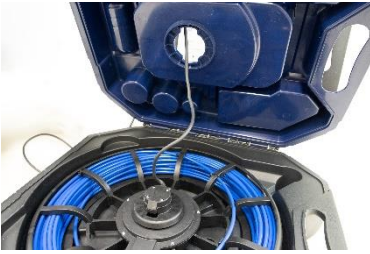
Fig. 60: Wrong: Camera cable not pulled tight
